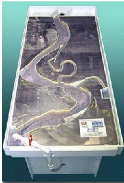
Micromodelo del río Mississippi (US Army Engineer District, Memphis, Corps of Engineers).
